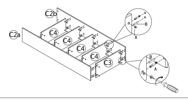
STEP 2: Insert the Dowel(B) to the Side Panel(C2a,C2b),Use a Phillips Head Screwdriver to insert the Cam Pin(A) to the Top Panel(C1),Assemble the Top Panel(C1) to the Side Panel(C2a,C2b),Use a Phillips Head Screwdriver to turn the Cam Lock(A)to lock onto the head of Cam Pin(A),Use Hex Key(F) to tighten the Leg(L)to the Bottom Panel(C3) with Bolt(C).
